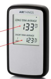
The radon screening device in this kit is called a Corentium Home, by Airthings. It is an electronic device that measures radon. Your device may look slightly different
